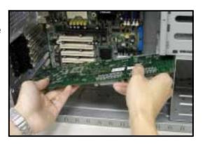
When the card is inside the chassis, push down the end of the card until it is level with the PCI slot.
